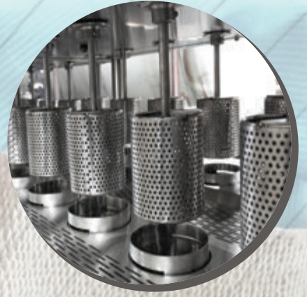
Kumaşa zarar vermeyen döner tambur (Tüylendirmeyen) Rotating drum that prevents fabric damage (Prevents Lint)
